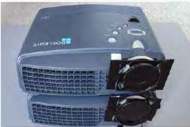
**3** Set up your two projectors with polarized filters. The filters are offset by 90 degrees
